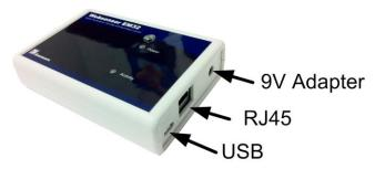
Figure 5a – Location of RJ45 and Wall Supply connectors.
